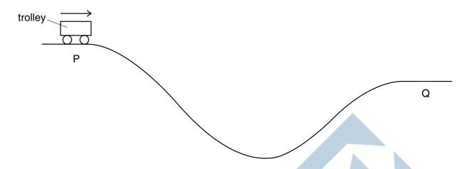
At P, the kinetic energy of the trolley is 5 kJ. Between P and Q the work the trolley does against friction is 10 kJ. Silation
