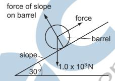
A force is applied to the barrel to move it up the slope at constant speed. The force is parallel to the slope.
