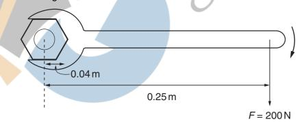
A force F is applied at right-angles to the spanner at a distance of 0.25 m from the centre of the nut. When the nut is fully tightened, the applied force is 200 N.
