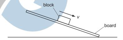
Which row describes the forces acting on the block when sliding with constant velocity?
