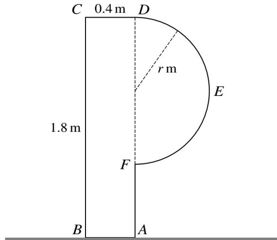
The diagram shows the cross-section  $ABCDEF$  through the centre of mass of a uniform prism which rests with  $AB$  on rough horizontal ground.  $ABCD$  is a rectangle with  $AB = CD = 0.4 \text{ m}$  and  $BC = AD = 1.8 \text{ m}$ . The other part of the cross-section is a semicircle with diameter  $DF$  and radius  $r \text{ m}$ .
