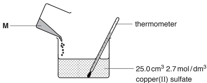
The student repeats the experiment using different masses of metal **M** and in each case calculates and records the maximum temperature rise.
