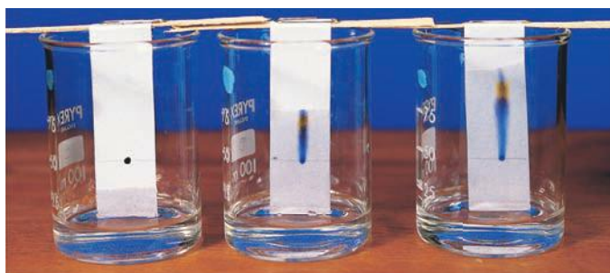
a Chromatographic separation of black ink.
