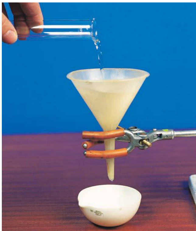
Figure 8.11 The excess magnesium is filtered in this way.
