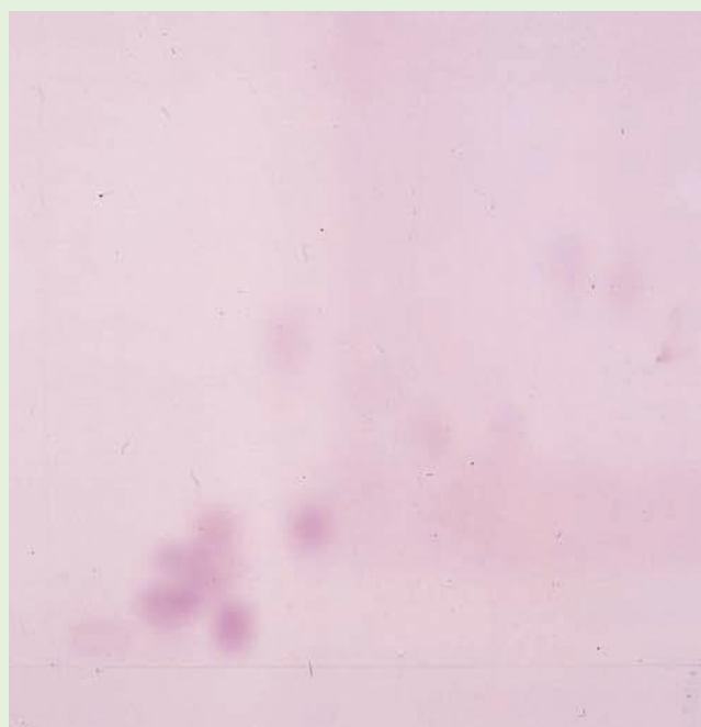
Figure 15.24 Amino acids can be separated and identified by TLC.
