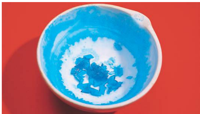
Figure 8.15 After slow evaporation to concentrate the solution, the solution is left to crystallise. Crystals of copper(II) sulfate are produced.
