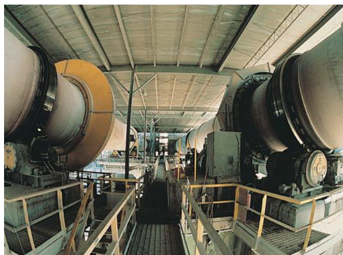
Figure 13.5 A modern rotary kiln.
