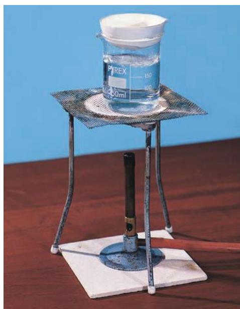
Figure 2.16 Apparatus used to slowly evaporate a solvent.
