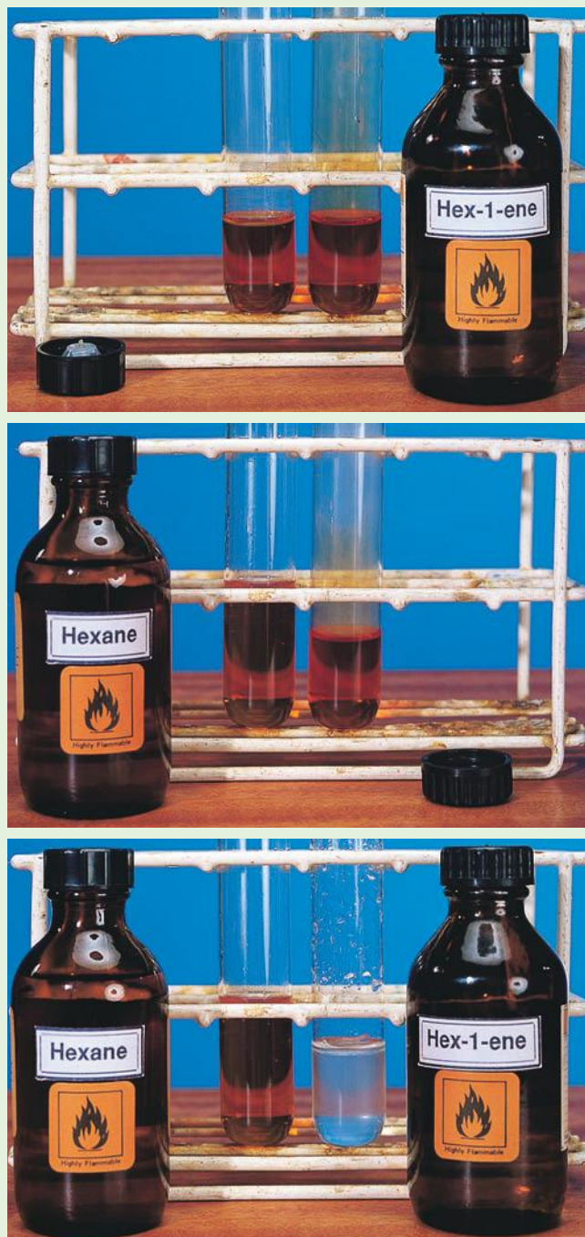
Figure 14.13 The alkene decolourises bromine in 1,1,1-trichloroethane.
